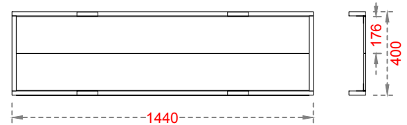
SOIL BOX WITH MECHANISED DROP. VIEW FROM UNDERNEATH
